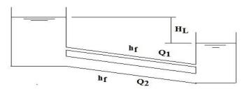
The friction losses through all pipes are the same, and all pipes discharge water independently.
