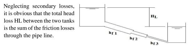
Friction losses through the pipe line are the sum of friction loss of each pipe. HL = hf 1 + hf 2 + hf 3 + ....
